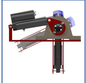
Image shows how the unit rotates based on controller inputs.
